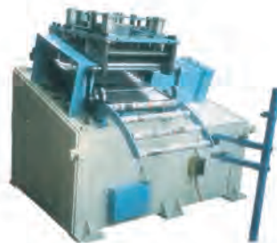
Precision Straightener with Backup Rolls & Cardan Shaft Arrangement
