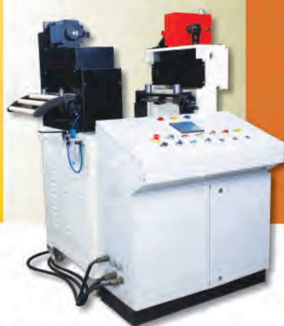
Transformer Lamination Punching, Notching & Variable Cut to Length Line
