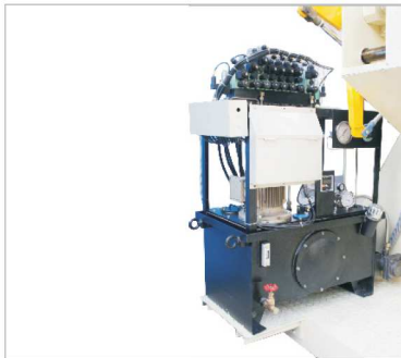
Hydraulics and Valve Arrangement
