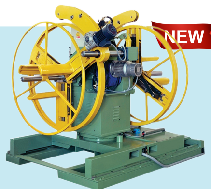
Dual Decoiler along with Hydraulic Jaw Expansion, Holddown and Disc Breaking Arrangement for 60 MPM line speed MDD-3000
